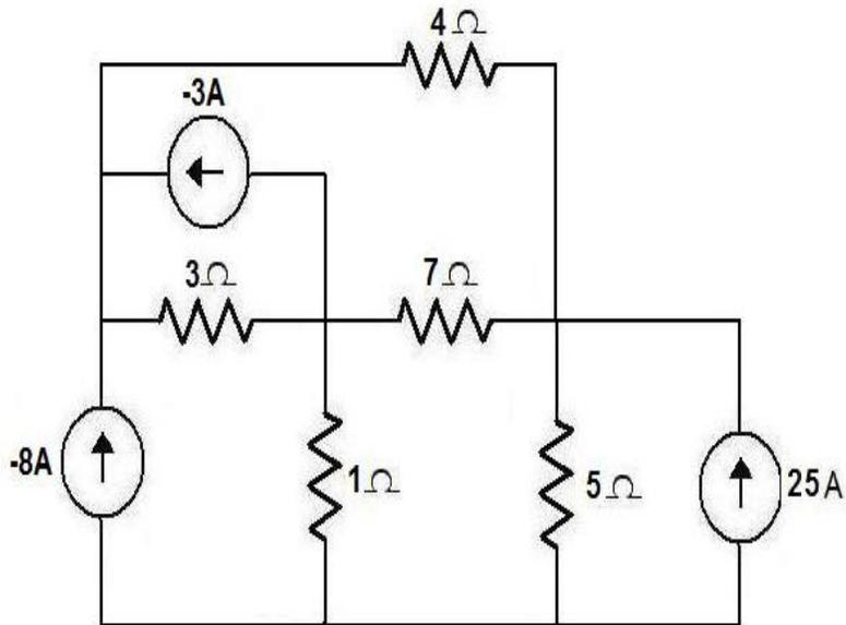
27. Using Mesh analysis, find current through 4 ohm resistor. (16)
